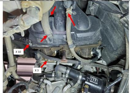
7. FROM UNDER THE DRIVER FENDER WELL, REMOVE THE AIR FILTER COVER AND AIR FILTER.
